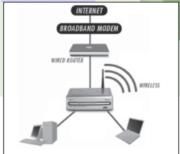
Remember also that each of your computers must have an Ethernet adapter. One cable will run from each computer to the switch and another cable will connect the switch to the modem/router. The LAN we just described is pictured in the above diagram. If you have questions or need help, give us a call.
